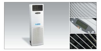
10 kW fan coil unit can connect to your existing chilled water circuit or to an Andrews packaged water chiller, heat pump or boiler. These units are fitted with fan speed controllers and internal condensate pumps.
