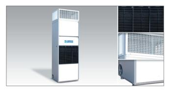
15 kW fan coil unit can connect to your existing chilled water circuit or to an Andrews packaged water chiller, heat pump or boiler. These units are fitted with fan speed controllers and internal condensate pumps.
