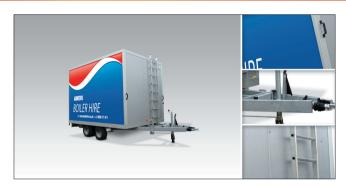
The 375 kW trailer mounted boiler, provides a fast efficient solution to a wide range of applications that require heating and hot water. This mobile boiler is housed in a sturdy vandal proof aluminium container mounted on a high speed trailer and is capable of delivering from 250 kW to 375 kW safely and efficiently.
