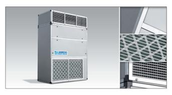
50 kW air handling unit can connect to your existing chilled water circuit or to an Andrews packaged water chiller, heat pump or boiler. These units are fitted with fan speed controllers and internal condensate pumps.
