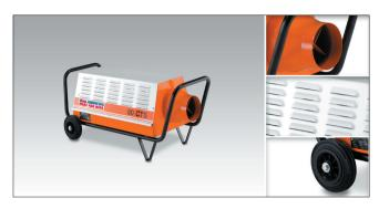
The CT80 has been designed to supply heat to awkward areas where access is difficult and can be fitted with up to 5 metres of flexible ducting. The CT80 is only available as a 415 volt 3 phase version with an output of 20 kW has an integral automatic control thermostat and a double skin construction to ensure low surface temperature.
