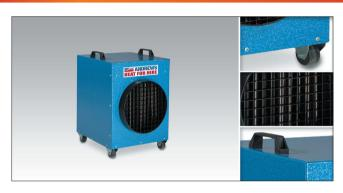
The DE95 is a very efficient electric fan heater and is available as a 415 volt 3 ph version only. The unit has three settings, 10 kW, 15 kW or 20 kW and can either be hard wired or supplied with a short cable tail and suitable plug. For automatic operation, the DE95 can be used in conjunction with the T32 control thermostat.
