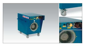
The ESH 20/40 fan assisted heater is designed for applications that need a large amount of electrical heating. The unit is only available in a 3 phase 415 volt version. The high pressure, high capacity fan enables the ESH 20/40 to deliver 40 kW of heat through ducting of up to 15 metres in length.
