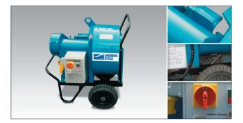
The FV300 ventilation/extraction fan is a robust high powered fan, used with ducting for the removal of dangerous fumes, dust particles and vapours. The FV300 has a maximum-ducted length of 40mtr and can be linked to heaters, boilers and chillers to distribute warm or cool air over large areas. The FV300 runs on 110 volt power supply.
