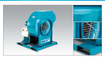
The FV600 ventilation/extraction fan is a robust high powered fan, used with ducting for the removal of dangerous fumes, dust particles and vapours. The FV600 has a maximum-ducted length of 40 metres and can be linked to heaters, boilers and chillers to distribute warm or cool air over large areas. This unit requires a 415 volt 3 ph power supply.
