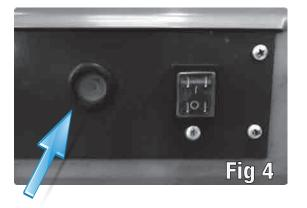
If the heater is allowed to run out of fuel the lockout light will illuminate. Replenish fuel supply and press reset button.
