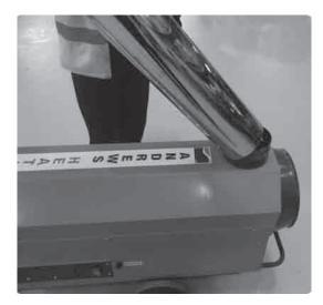
**Fig 1 :** Fit warm air supply duct if required. Maximum 6 mts x 300 mm dia.
