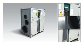
The KT6000 desiccant dehumidifier, is best used where the work is being carried out at very low temperatures and very low relative humidity is required. The KT6000 desiccant dryer is more efficient than refrigerant dryers at about -5°C. This unit requires a 415 volt 3 ph power supply.
