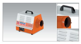
The CT20 has been designed to supply heat to awkward areas where access is difficult and can be fitted with up to 3 metres of flexible ducting. The CT20 is only available as a 230 volt version; has an integral automatic control thermostat and a double skin construction to ensure low surface temperature.
