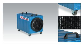
The DE65 is a very efficient electric fan heater and is available as a 415 volt 3 ph version only. The unit has three settings, 6.5 kW, 9.5 kW or 13 kW and can either be hard wired or supplied with a short cable tail and suitable plug. For automatic operation, the DE65 can be used in conjunction with the T32 control thermostat.
