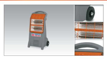
Designed to achieve local 'spot' heating within large areas. The Quartz heats up within seconds and delivers up to 3 kW of heat from the two infra-red emitters. The radiant Quartz runs on 110 or 230 volt power supply.
